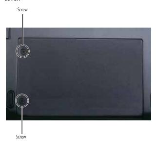
11 Remove the two hard drive screws.
