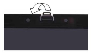
4 Close the LCD panel onto the keyboard. There is a click when the LCD panel latch locks.
