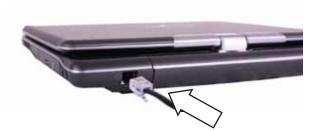
Insert the other end of the modem cable into a telephone wall lack.
